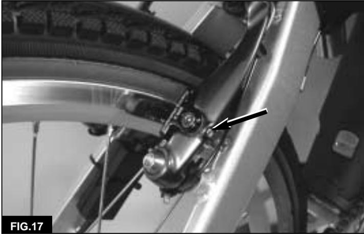
Small changes in the modulation adjustment can have a significant effect upon brake pressure and stopping ability. Whenever you adjust the modulation, adjust each caliper in 1/4 turn increments and test the brakes. Always adjust each side of the brakes equally. If you increase the modulation on the left caliper by 1/4 turn, you should also increase the modulation on the right caliper by an equal amount.
