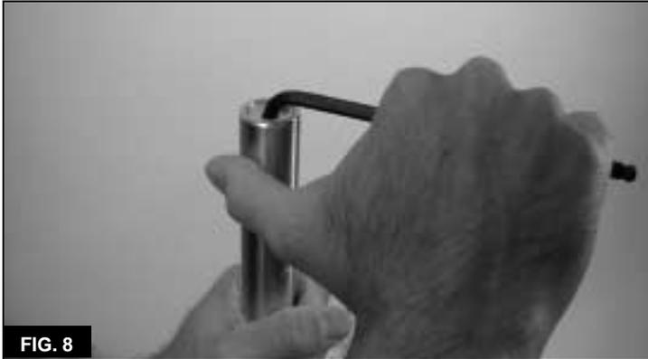
2. Turn the side-to-side adjuster (**A, Figure 7**) in or out to adjust the amount of side-to-side play at the saddle tip.
