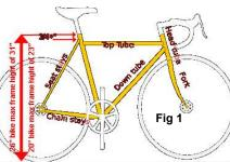
Bottom of GoBike Rack must sit between 1 and 2 inches above the rear tire.
