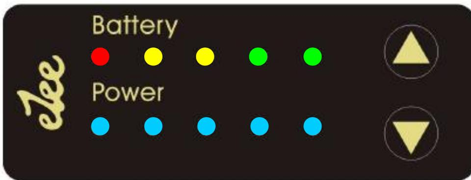
**Battery level** shows the state of charge of the battery. As you continue to cycle and the battery power drops, the level gauge will correspond to the state of charge remaining. If the battery level shows red, it is nearly empty.
