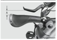
Before every ride, carry out a stationary brake test. To do so, pull the brake levers towards the handlebar using two fingers and normal braking force. The brake lever must not come into contact with the handlebar (▷ page 24). A distance "A" must remain between the brake lever and the handle, even when maximum hand force is applied.
